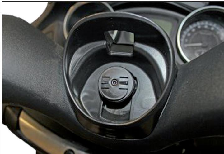
**GB** Support mounted on the handlebar.
