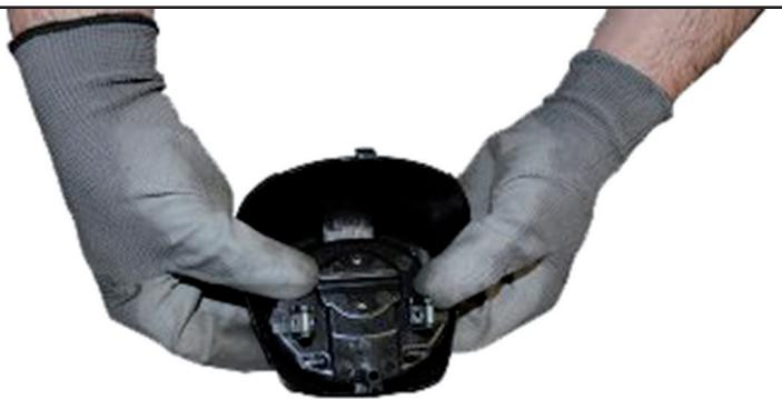
**GB** Line up the holes of the screws that were removed with those on the support.
